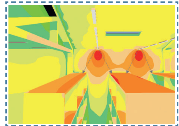
Side view high bay corridor with shelving 12m Emed. Floor 156 lux Uniformity 0.62
